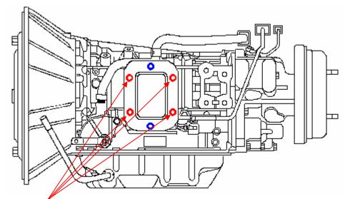
THESE FOUR (4) BOLT HOLES ARE DRILLED THROUGH. DO NOT INSTALL THE THREADED PORTION OF A PTO MOUNTING STUD OR BOLT IN EXCESS OF A DEPTH OF 15mm OR INTERNAL DAMAGE MAY OCCUR.
