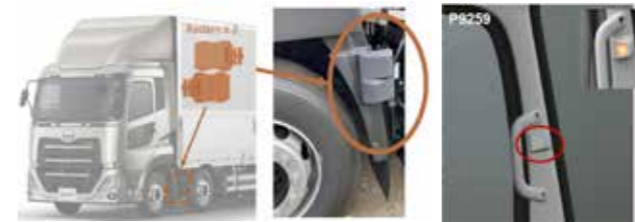
Smart BSIS and Smart LCS radars location on the QUON
